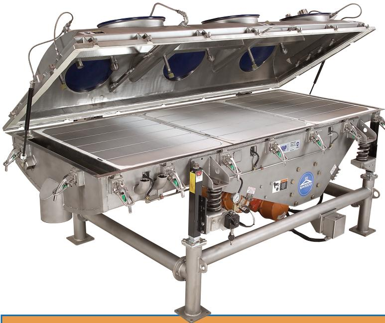
The V3 Rectangular Separator has many advantages adding to its flexibility and versatility as a high-volume screener. The V3's deck angle can be inclined or declined at a range of 5° to maximize the effectiveness of the system. Furthermore, all accessories available with other rectangular separators are accessible with the V3, including self-cleaning screens, vibrating spray systems, spray balls, misting nozzles, acid washdown, and vibrating covers.
